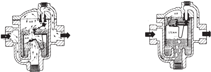
Fig. 18-1— Thermic bucket operation. At left, thermic vent is open and air “passes” through. At right, thermic vent is closed and trap operates same as a standard trap.
