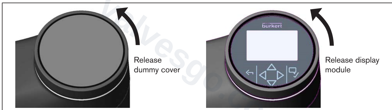
Figure 24: Removing dummy cover or display module
