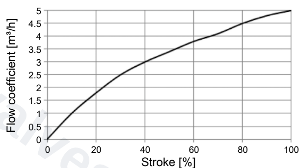
Fig. 21: Actuator size 70 (M), flow characteristic DN15
