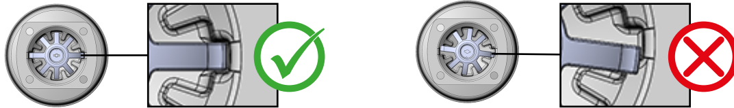
Fig. 34: Correct and incorrect position of the compressor
