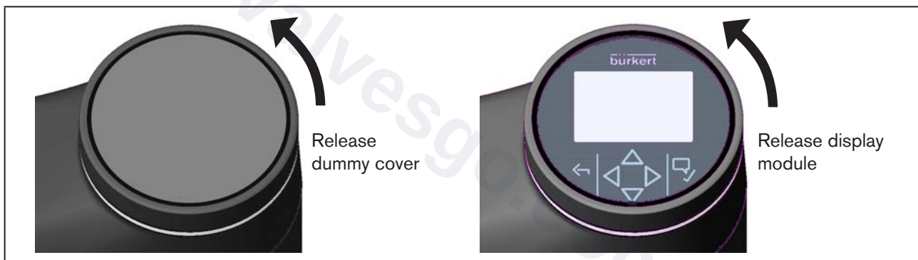
Figure 27: Removing dummy cover or display module
