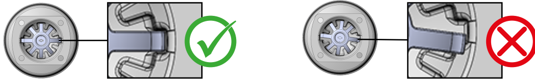
Fig. 34: Correct and incorrect position of the compressor
