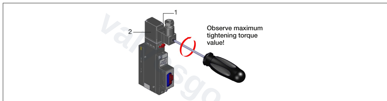
Figure 9: Connection of the cable plug
