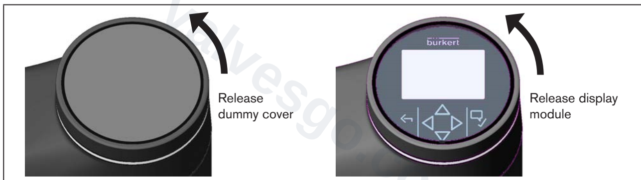
Figure 24: Removing dummy cover or display module
