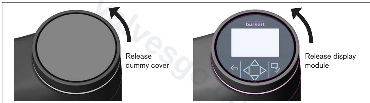
Figure 24: Removing dummy cover or display module
