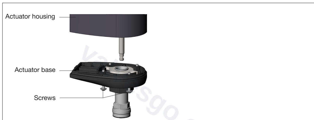
Fig. 13: Removing actuator housing from the actuator base
