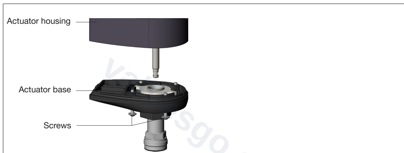
Fig. 13: Removing actuator housing from the actuator base
