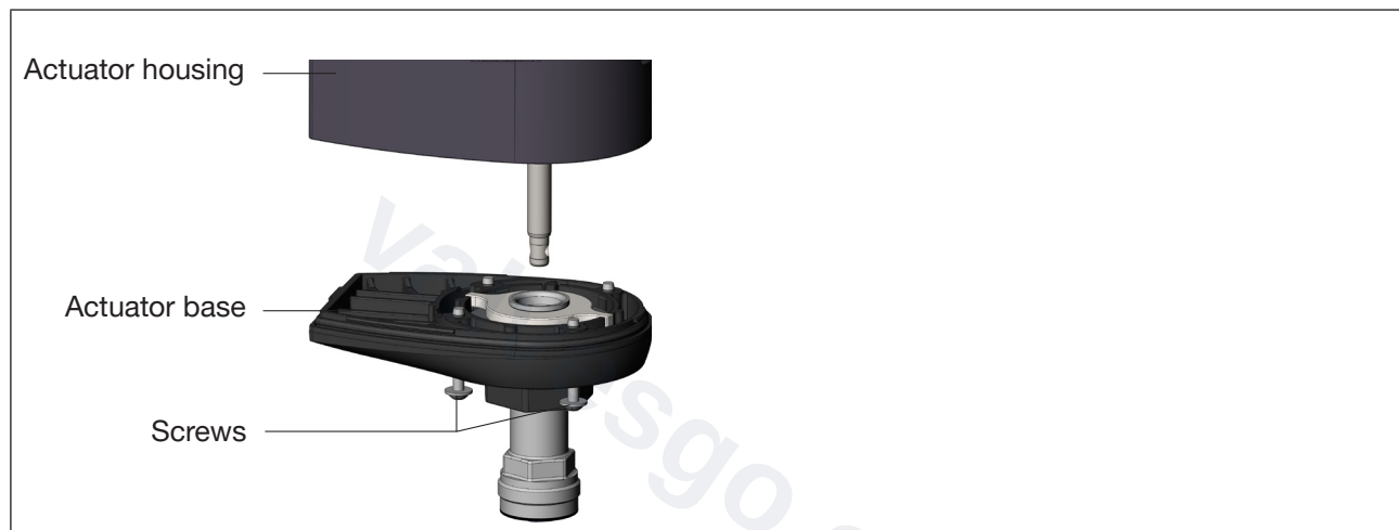
Fig. 13: Removing actuator housing from the actuator base
