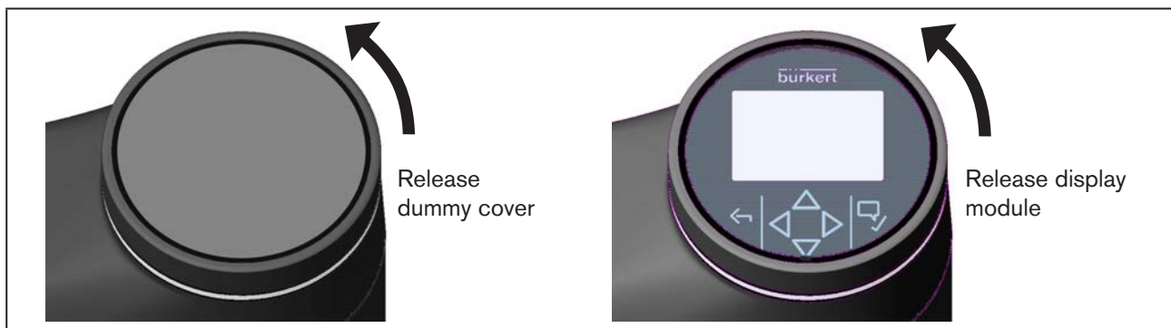
Figure 24: Removing dummy cover or display module
