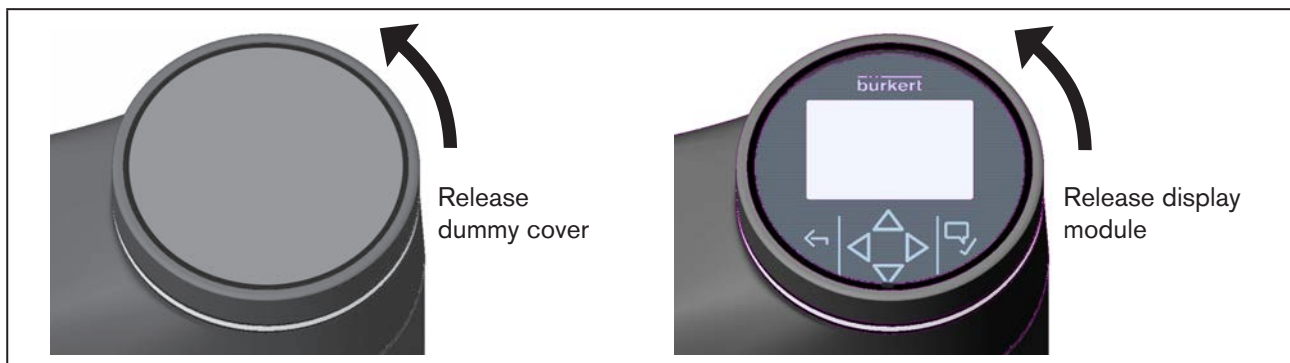
Figure 15: Removing dummy cover or display module
