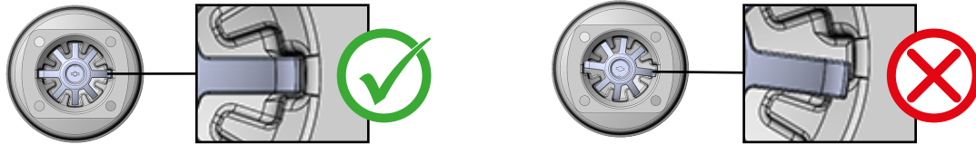
Fig. 18: Correct and incorrect position of the compressor
