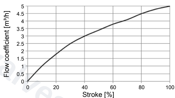
Fig. 21: Actuator size 70 (M), flow characteristic DN15
