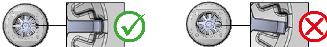
Fig. 25: Correct and incorrect position of the compressor
