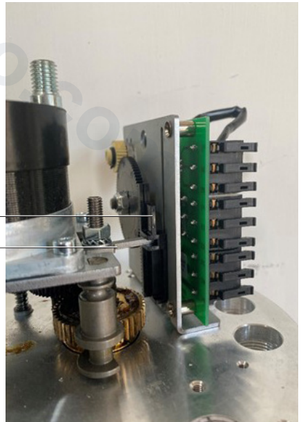
Fig. 8 Auxiliary Travel Switch (WE) Feedback Arrangement (1-6 kN)
